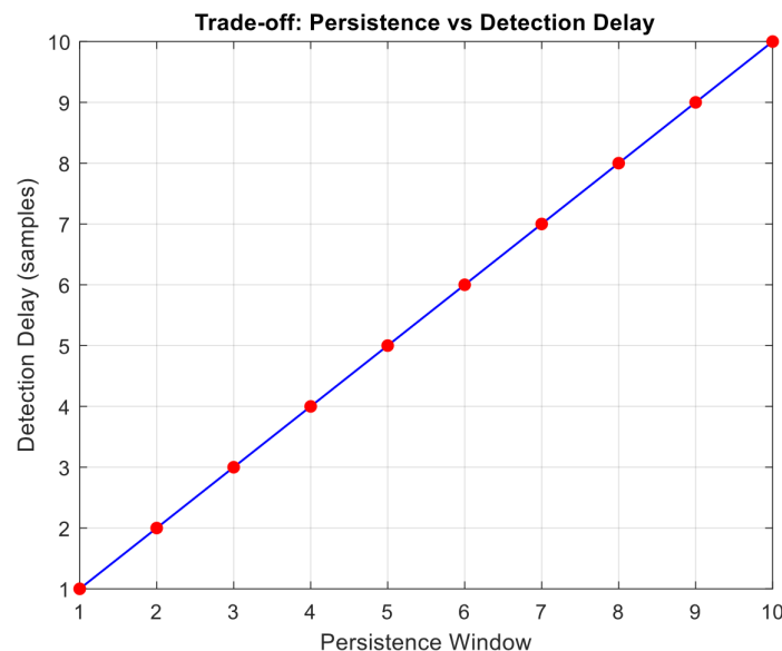
Figure 5. Detection Delay vs Persistence Window
